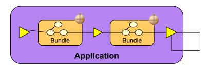
OSGi Bundles assembled in an OSGi Application and integrated through services in the OSGi service registry
