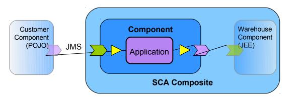
SCA Composite assembled from heterogeneous components including an OSGi Application component, and integrated through SCA services with configurable bindings (JMS, web services...).
